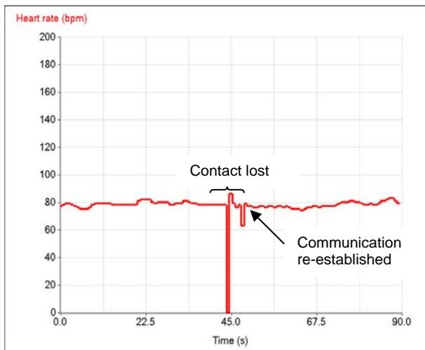
If the finger/earlobe clip 'loses contact' with the pulse, the reading may momentarily drop to zero.
