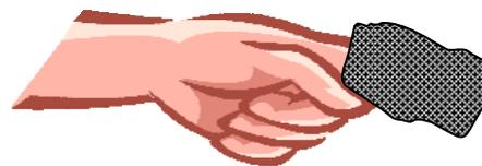
The light sensitive detector (LSD) in the clip can be sensitive to high levels of ambient infrared light e.g. bright sun or room lights. If the light interferes with the detector the Sensor may 'lose contact'. Stop logging, and reduce the light level e.g. by covering the sensor clip before starting to log again.
