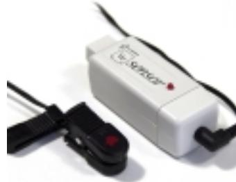
The Heart Rate sensor sensing clip (pleth) holds an infrared LED that shines a light through either a finger or ear lobe onto a light sensitive detector. As the amount of light transmitted varies with the flow of blood, the sensor can record either blood flow (heart waveform), or heart rate (beats per minute).
