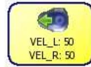
Another important option when configuring motors is the "**Wait until end of command**". This option allows you to block the movement command (the program stops running) until the movement module finishes (according to time or distance). This option is only accessible if we select the options "Enable end according to time" or "Enable end according to distance".
