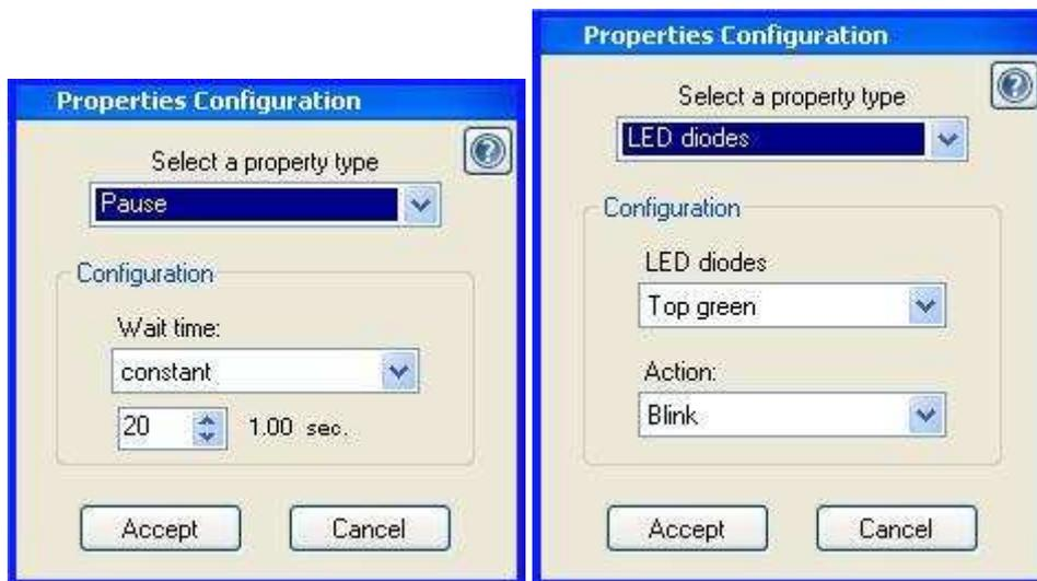
**Image 63. Pause and LEDs configuration**
