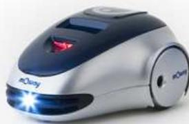
**Image 15. Robot with Front LED and red LED switched on**
