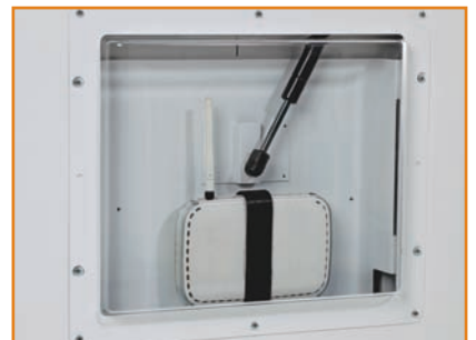
Optional Wifi module for mounting a wireless access point inside the Perspex bubble, enabling greater reception as well as a clear view of the connectivity status at all times.
